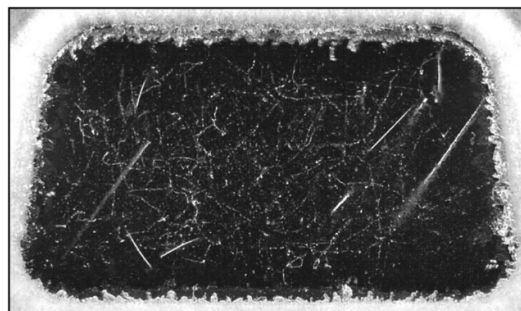
Figure 3. A composite image of hundreds of cosmic ray tracks. Electrons, muons and protons can be distinguished by the appearance of their tracks. Typically, tracks are visible at a rate of about one per second.
