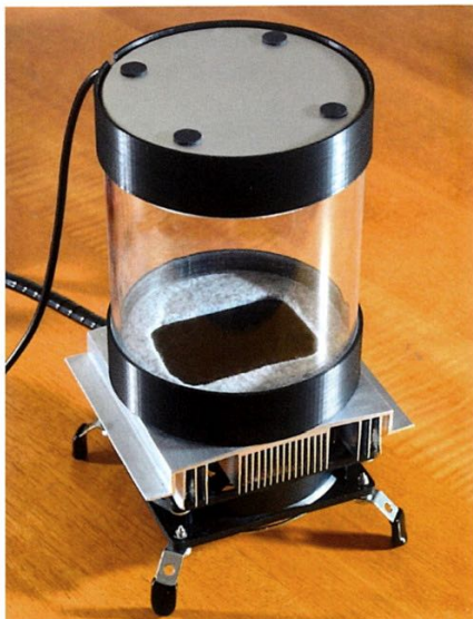
◀ The cloud chamber comprises a glass or plastic jar with a heater at the top and a small refrigeration unit at the bottom. All the essential components of the design are readily available from online retailers.
