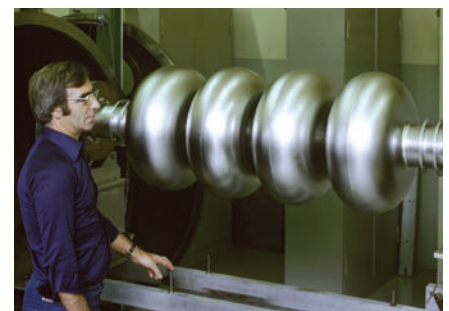
RF cavity. Typically a few meters long, it sustains accelerating rates of ~0.1 GeV/m. © CERN.
