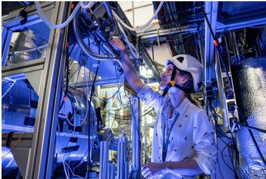
BASE physicist Barbara Latacz in front of the experiment's cryostat. This cylinder, which is kept at 4 kelvins (-269°C), houses the system of traps that cool and measure the antiprotons and a very strong magnet. (Image credit: CERN)
