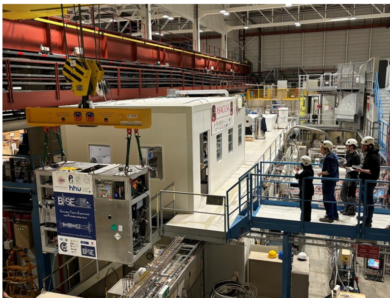
The BASE-STEP transportable trap system, lifted by crane through the AD hall before being loaded onto a lorry. The team monitored all the parameters during transport. (Image credit: CERN)
